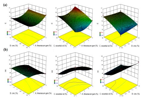
Figure 2: Response surface plots for the effects of Carboxymethyl Cellulose (CMC), Amuniacum Gum (AMG), and Clove Essential Oil (CEO) in composite films on color properties for total color difference ( $\Delta$ E) (**a**), and Whiteness Index (WI) (**b**)
