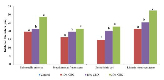
**Figure 6:** Antibacterial activity of the enriched Carboxymethyl Cellulose (CMC)-Amuniacum Gum (AMG) film with Clove Essential Oil (CEO). Different letters (a–c) indicate the significant differences (p<0.05). Values are expressed as mean±standard deviation
