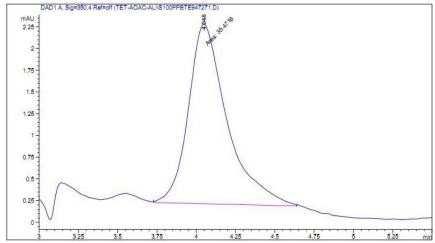
Figure 3: The High-Performance Liquid Chromatography (HPLC) of the mixed standard solution of tetracycline (100 ng/g)
