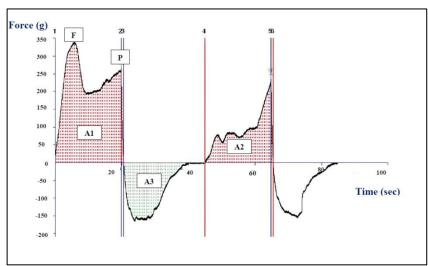
**Figure 3**: Texture profile Analysis (TPA) curve for camembert cheese made from 100% cow milk. The calculation of textural properties: P=Hardness (N); F=Fracturability (N); A<sub>2</sub>/A<sub>1</sub>=Cohesiveness; A<sub>3</sub>=Adhesiveness (g·s); Chewiness=hardness×cohesiveness×springiness (N)
