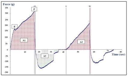
Figure 4: Texture profile Analysis (TPA) curve for camembert cheese made from 90% cow milk and 10% buttermilk. The calculation of textural properties: P=Hardness (N); F=Fracturability (N);  $A_2/A_1$ =Cohesiveness;  $A_3$ =Adhesiveness (g·s); chewiness=hardness×cohesiveness×springiness (N)
