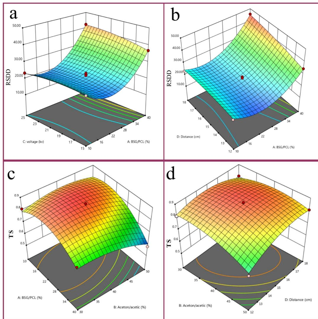
**Figure 1:** The independent variables' interaction and effect on the dependent variables. (a): The interaction effect of variables Basil Seed Gum (BSG%) and voltage on the Relative Standard Deviation of nanofiber Diameter (RSDD); (b): The interaction effect of variables BSG% and distance on RSDD; (c): The interaction effect of variables BSG and acetone% on Tensile Strength (TS) of nanofibers; (d): Interaction effect of two variables acetone% and distance on TS of nanofibers.
