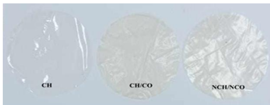
Figure 2: Images of chitosan film (CH), and chitosan-collagen composite film (CH/CO), and chitosan-collagen nanocomposite film (NCH/NCO)
