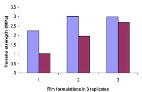
Fig. 2: Tensile strength of two different film formulations measured by Instron
