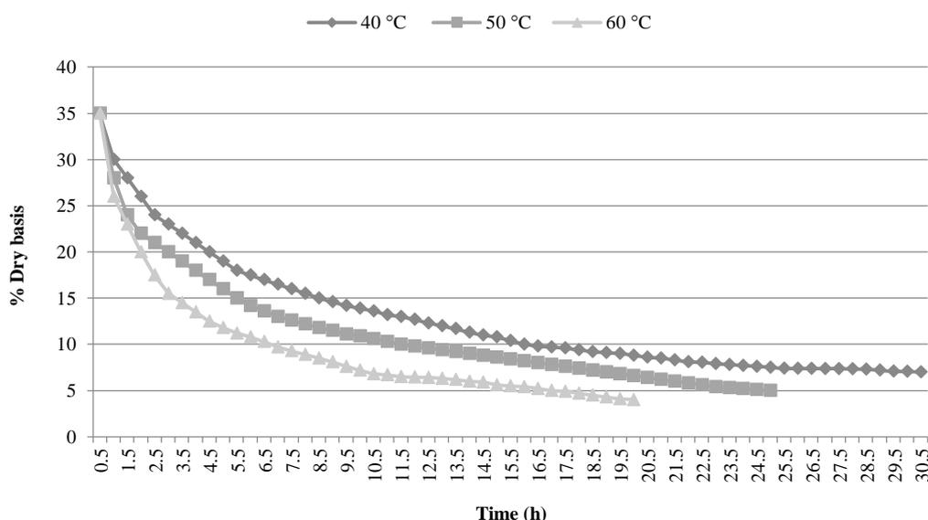
**Figure 2:** Moisture content reduction of hazelnuts over time at different temperatures (40, 50, and 60 °C)
