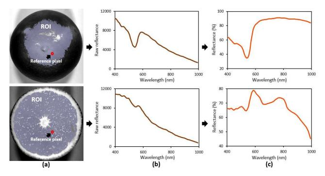
Figure 1: Main steps for image and spectra processing of orange fruit: (a) identification of the Region of Interest (ROI), (b) raw mean reflectance spectrum, and (c) corrected reflectance
