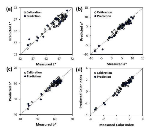
Figure 5: Observed versus predicted values of external quality attributes using simplified models: (a) L\* parameter, (b) a\* parameter, (c) b\* parameter, and (d) color index
