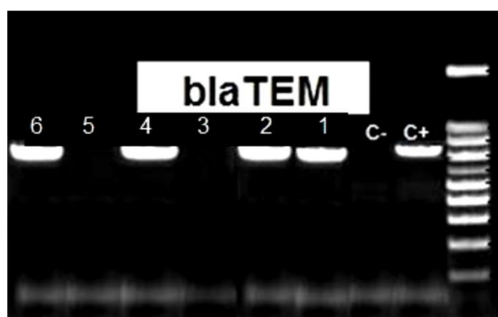
Figure 2: Agarose gel electrophoresis of bla TEM Polymerase Chain Reaction products using 100 bp DNA ladder. Lane C+: positive control; lane C-: negative control; lanes 1, 2, 4, and 6: isolates with bla TEM genes; lanes 3 and 5: isolates without bla TEM gene.
