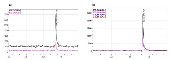
Figure 1: Liquid Chromatography-Tandem Mass Spectrometry (LC-MS/MS) chromatogram of acrylamide fragment ions m/z 55.0 and 27.20 in raw potato spiked at level of 60  $\mu$ g/kg acrylamide (a: left side) and Acrylamide-d3 (AAd3) fragment ions m/z 58.15 and 30.10 in raw potato spiked at level of 500  $\mu$ g/kg AAd3 (b: right side)
